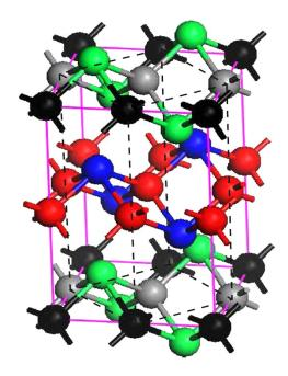
FIG. 1 (color online). The  $Q_M$  antiferromagnetic structure of LaFeAsO, with different shades of Fe atoms (top and bottoms planes) denoting the opposing directions of spins in the  $Q_M$  AFM phase. Fe atoms lie on a square sublattice coordinated tetrahedrally by As atoms, separated by LaO layers (center of figure) of similar structure. The dashed lines indicate the non-magnetic primitive cell.
