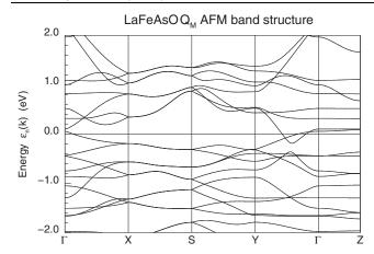
FIG. 3. Band structure of the  $\vec{Q}_M$  AFM phase along high symmetry directions. Note that two dispersive bands and one narrow band cross  $E_F$  along  $\Gamma$ -Y, while only the one flatter band crosses  $E_F$  (very near k=0) along  $\Gamma$ -X.
