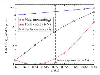
FIG. 5 (color online). The magnitude of the Fe magnetic moment, the change in energy, and the Fe-As distance, as the As height  $z_{\rm As}$  is varied.
